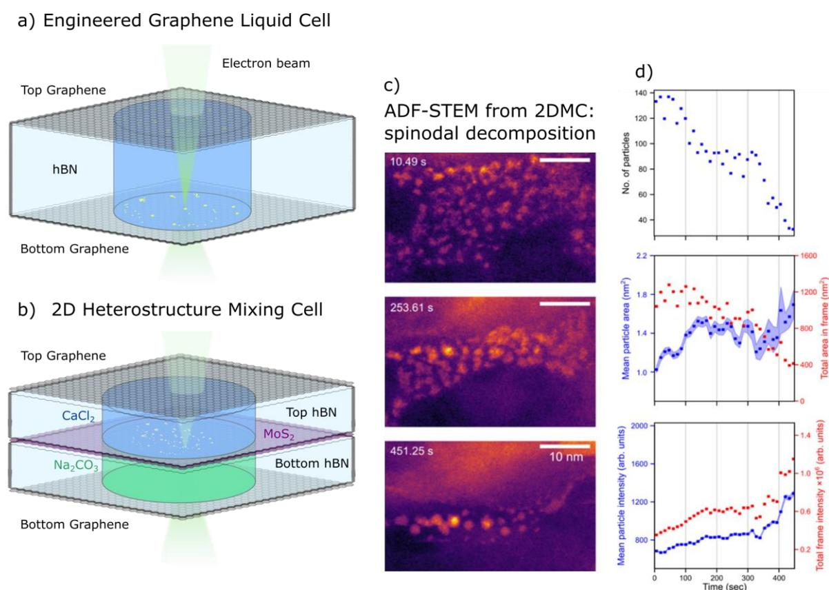
Figure 1: Schematic of a) engineered graphene liquid cell and b) two-dimensional heterostructure mixing cell, each with annotated components. c) Annular dark field scanning transmission electron micrograph series showing CaCO<sub>3</sub> formation. d) Size, morphology and density analysis of species visible in c)
