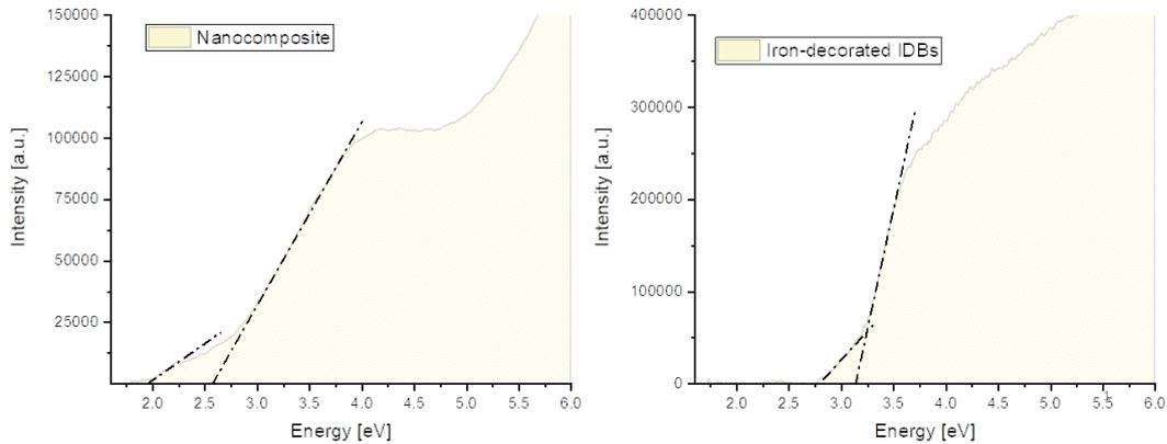
**Figure 1.** *Left:* EELS spectrum from a single ZnFe<sub>2</sub>O<sub>4</sub> nanoparticle in bulk ZnO. *Right:* EELS spectrum from the sample containing iron-decorated IDBs.
