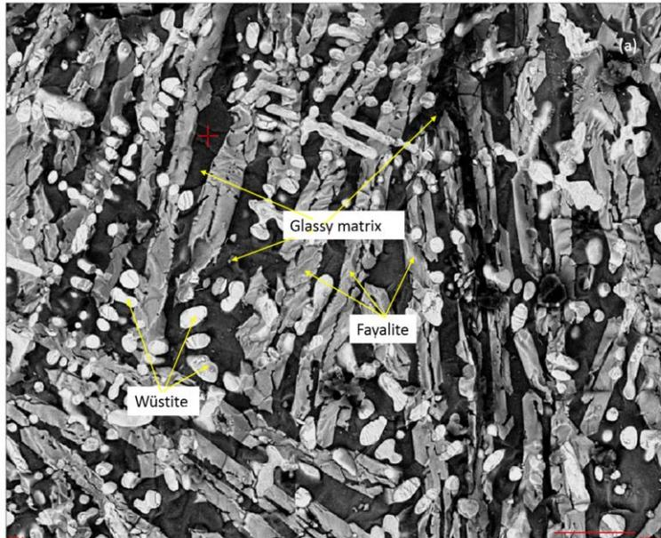
Figure 1. BSE image of the microstructure of an iron smelting slag sample indicating its main components from an archaeometallurgical investigation
