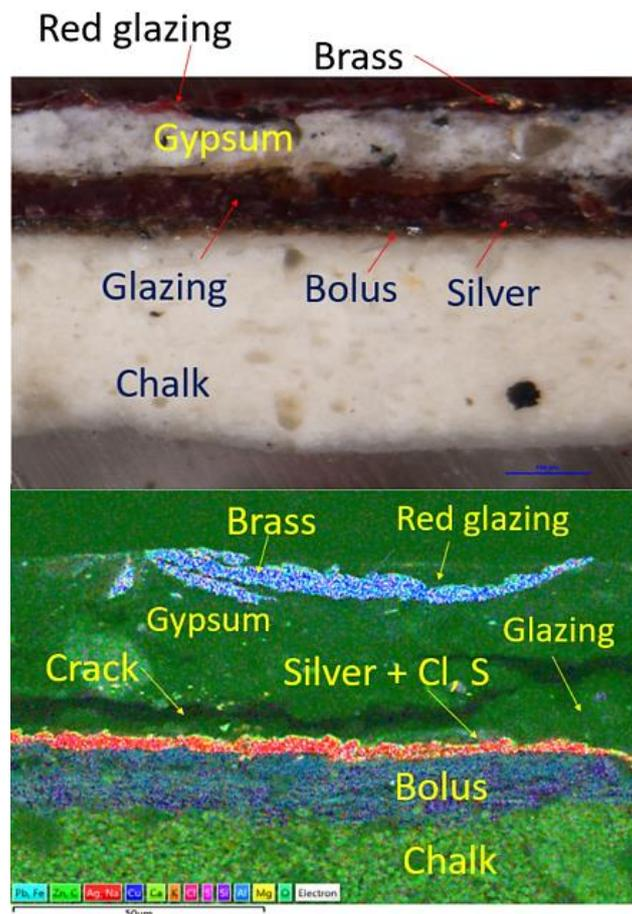
Figure 2. Optical micrograph (top) and overlaid EDS elemental mapping (bottom) of a sample from a polychrome sculpture displaying the original materials in the lower layers with a silver applied in a water gilding method along with signs of deterioration products, and materials introduced due past conservation interventions in the upper layers.
