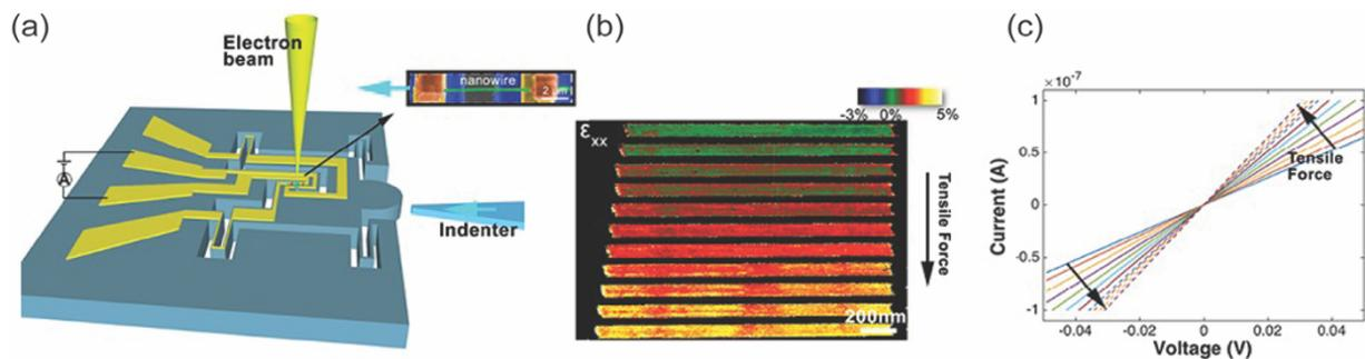
Figure 1. An example of the in situ TEM measurements on individual nanowires: (a) A schematic of an experimental setup used for the study. Tensile stress can be applied on a nanowire. Meanwhile, TEM, mechanical and electrical measurements are performed on the nanowire. (b) 4D STEM strain maps of the nanowire as a function of applied stress. (c) Changes in I-V characteristics of the nanowire due to applied stress.
