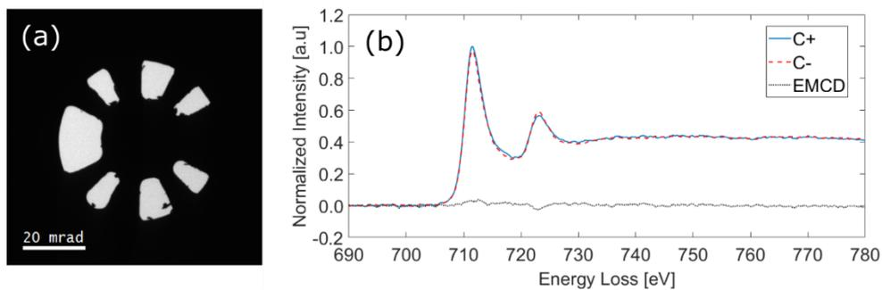
Figure 2. (a) The mirrored ventilator aperture (VA) which can simultaneously acquire the positive and negative EMCD components in zone axis (b) the + and – EELS spectra and their difference (EMCD) signal acquired using the VA from an Fe sample in [001] zone axis with 5 mrad convergent electron probe.
